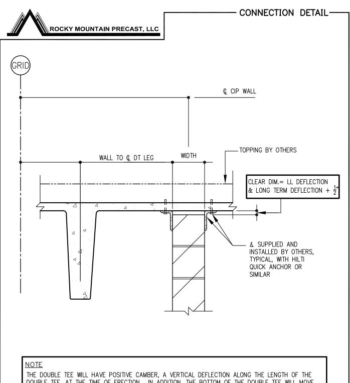
THE DOUBLE TEE WILL HAVE POSITIVE CAMBER, A VERTICAL DEFLECTION ALONG THE LENGTH OF THE DOUBLE TEE, AT THE TIME OF ERECTION. IN ADDITION, THE BOTTOM OF THE DOUBLE TEE WILL MOVE CONTINUALLY DUE TO TEMPERATURE CHANGE, CREEP AND VARIATIONS IN APPLIED LIVE LOAD. DUE TO THIS, THE BOTTOM OF THE DOUBLE TEE WILL NOT BE PARALLEL WITH THE TOP OF THE CAST—IN—PLACE WALL. THIS MAY BE OBJECTIONABLE IN APPEARANCE AND SHOULD BE CONSIDERED AT THE TIME OF DESIGN.
